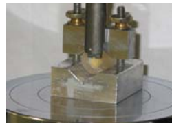
Figure 2: Shear Bond Test Set-Up
